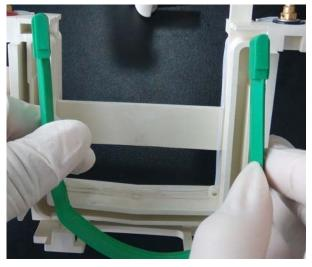
b. Rotate the gasket 180 degree and Installed it back oppositely (outside inwards, inside-out). Press down around with your thumbs using even pressure to ensure to seal well to prevent leakage.
